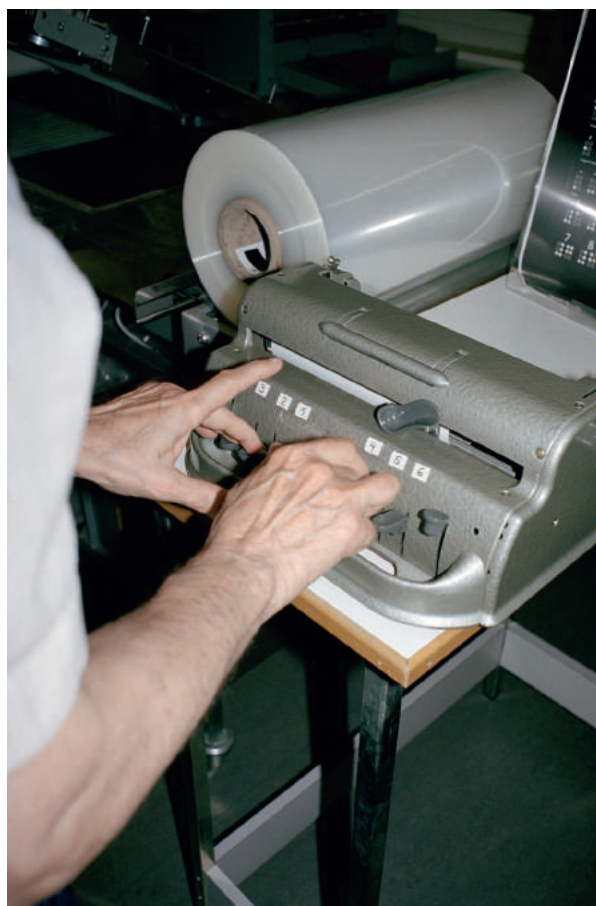
The Perkins is an old mechanical typewriter for Braille texts. It's like a ballpoint pen for the blind, René Moser explains during the demonstration.
